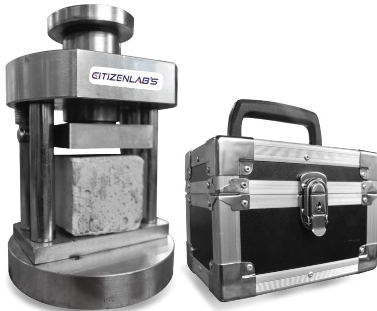
**MORTAR CUBE COMPRESSION DEVICE [50 mm (2")]**
