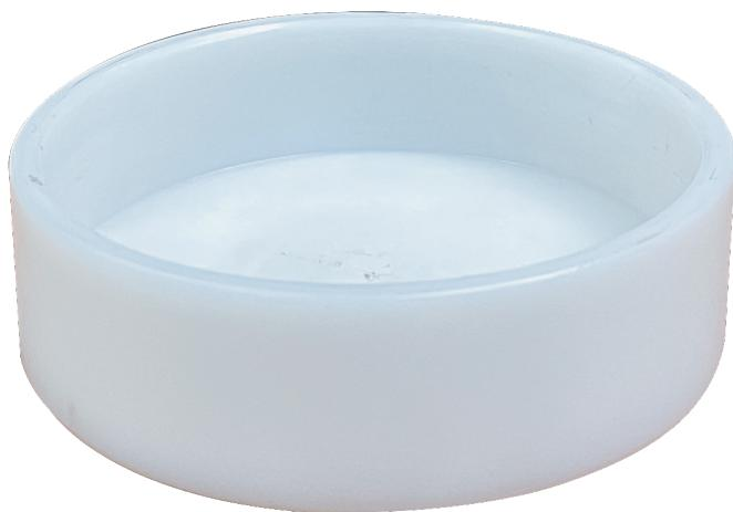
**MOULD FOR WATER RETENTION**
